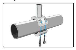
2. Slide the mounting plate onto the post and then tighten down the bolts.
