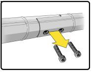
2. Replace with Black Quick Release Knobs. Repeat on each hinge section of tower. Place in front hole.
